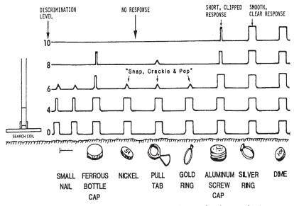
NOTE: The discrimination levels shown are typical values only and may vary from detector to detector. Figure 5. Typical 1280-X audio responses over 1 inch deep targets with search coil sweeping 1 to 2 inches above ground.
