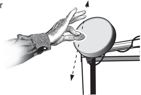
III. Click on detector with the left knob. Set the Gain at the 12:00 position for this demonstration.
