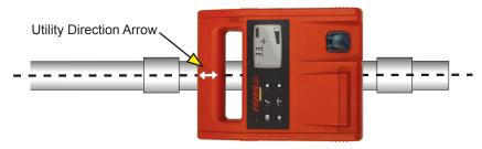
Figure 13. Inductive Coupling Tracing Alignment
