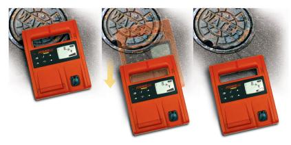
Keep large metallic objects away from the Transmitter handle when using the inductive mode. The energizing field is generated inside the handle of the Transmitter. A large metal object near the Transmitter handle will cause the Transmitter to "overload." In response to an overload condition, the Transmitter automatically lowers the power to a safe level and alerts the operator (with audio indicator and flashing overload symbol) to move the Transmitter to an alternate location.
