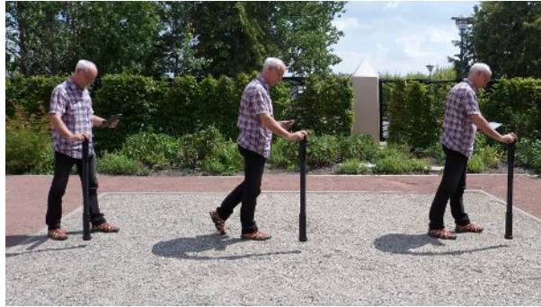
Figure 7.5: Probe should always point downwards and should not be turned
