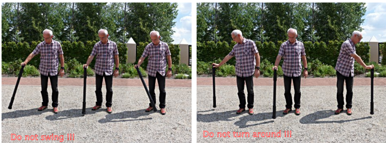
Figure 7.6: Pivoting or turning of the probe falsifies the measurement
