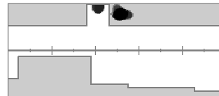
The Target Trace of a 1998 Canadian 10¢ coin (accepted) and a directly adjacent nail (rejected).
