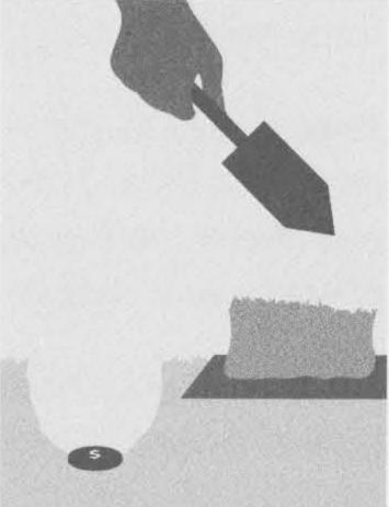
Check the hole for the target. If it is not in the hole, place the detector on the ground with the coil flat, pick up a handful of soil and pass it over the coil. Be sure not to wear rings, bracelets or a watch which will produce a signal. Repeat this procedure until the target is located.
