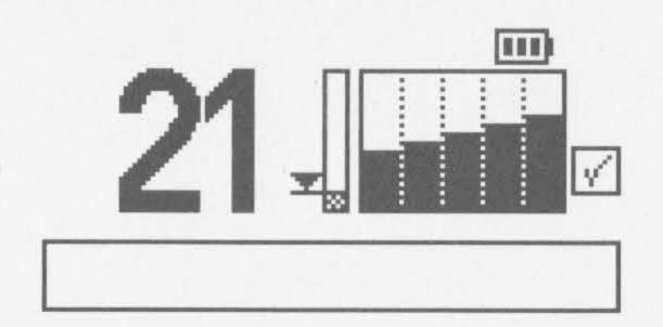
In Pinpoint, Safari will produce a clear 'beep' as the search coil passes directly over the target. The locator bar graph in the Detect Screen will also fill out on the screen as the coil passes directly over the target.
