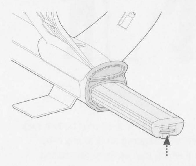
**5** Remove the battery pack entirely from the battery compartment.
