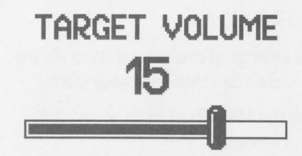
Target Volume can be used to prevent signals from large and shallow items producing very loud signals that are uncomfortable to your ears. This should be adjusted to suit your individual hearing.
