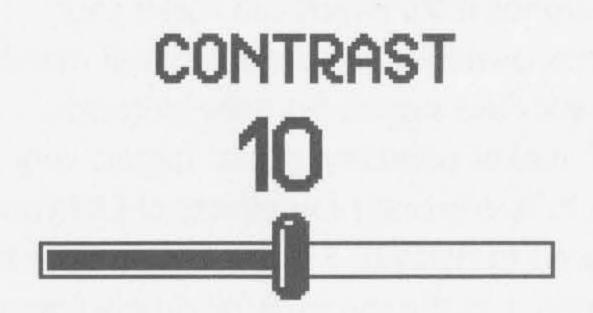
By adjusting the Contrast, relative to the current light conditions, you may make the information on the LCD easier to see.
