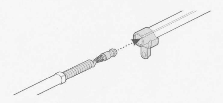
3 Slide the Upper Shaft over the Lower Shaft, so the coil cable appears out the top.
