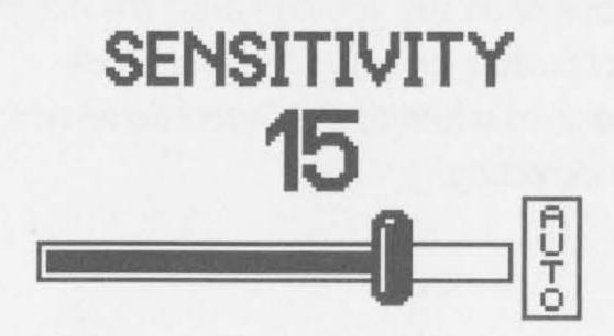
A manual Sensitivity setting can be used in areas with blanket/constant soil mineralisation, such as beaches or modern parks. However, Auto Sensitivity is the preferred setting when detecting areas with variable soil conditions, until you become experienced with your detector.
