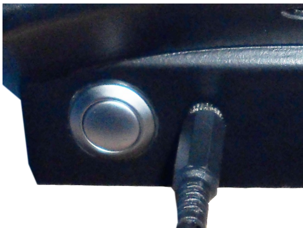
Illustration 5.4: Connection of joystick
