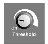
The Threshold control is also used to turn the detector on.
