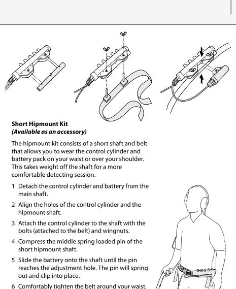
Ensure that you position the hipmount shaft in a way that does not cause excessive
