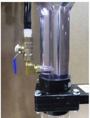
To set the drop water flow, watch the dirt in the trap. Slowly reduce the drop water flow on the meter. As you reduce the drop water flow, you will observe dirt dropping into the drop tube. Set the flow to allow some dirt to penetrate the drop tube ½ the length of the tube and observe the drop water reading.
