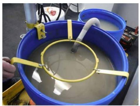
Place the tailings bucket support frame in the drum on your right by spreading the arms to hook over the edge of the drum. Place the tailings bucket in the frame. (see picture #2)
