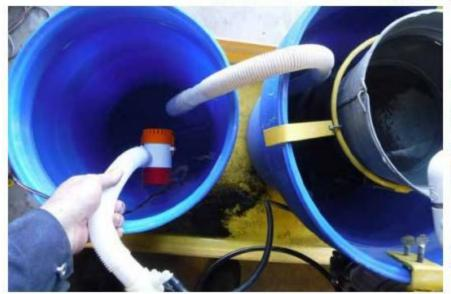
To the drum on your left (the pump drum), submerge the pump into the water and allow the pump to fill with water (do not submerge the clamps).
