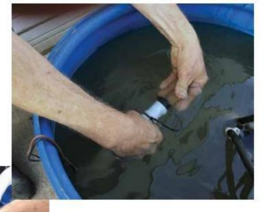
will cause the water to transfer by gravity from one bucket to the other keeping the bucket water levels equal. (see picture #5)
