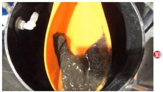
The pay dirt drops submerged into the Goldrop collection jar at the bottom of the unit. The Blow Out valve (see picture 11) is used to clear the trap of dirt into the tailings bucket and to help keep the paydirt in suspension during processing. Adjust this valve carefully during processing to keep the dirt in slight motion.
