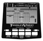
The complete operating status of your detector is shown on the screen at all times. When the TREASURE IMAGING (automatic pinpointing and sizing) touchpad is pressed and held, size and depth of targets will also be shown. The mode in which you are searching will always be shown on the left side of the screen under the SEARCH MODE heading.
