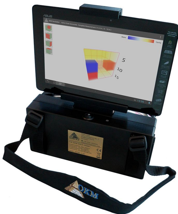
Figure 6.3: Tablet PC mounted to Controller
