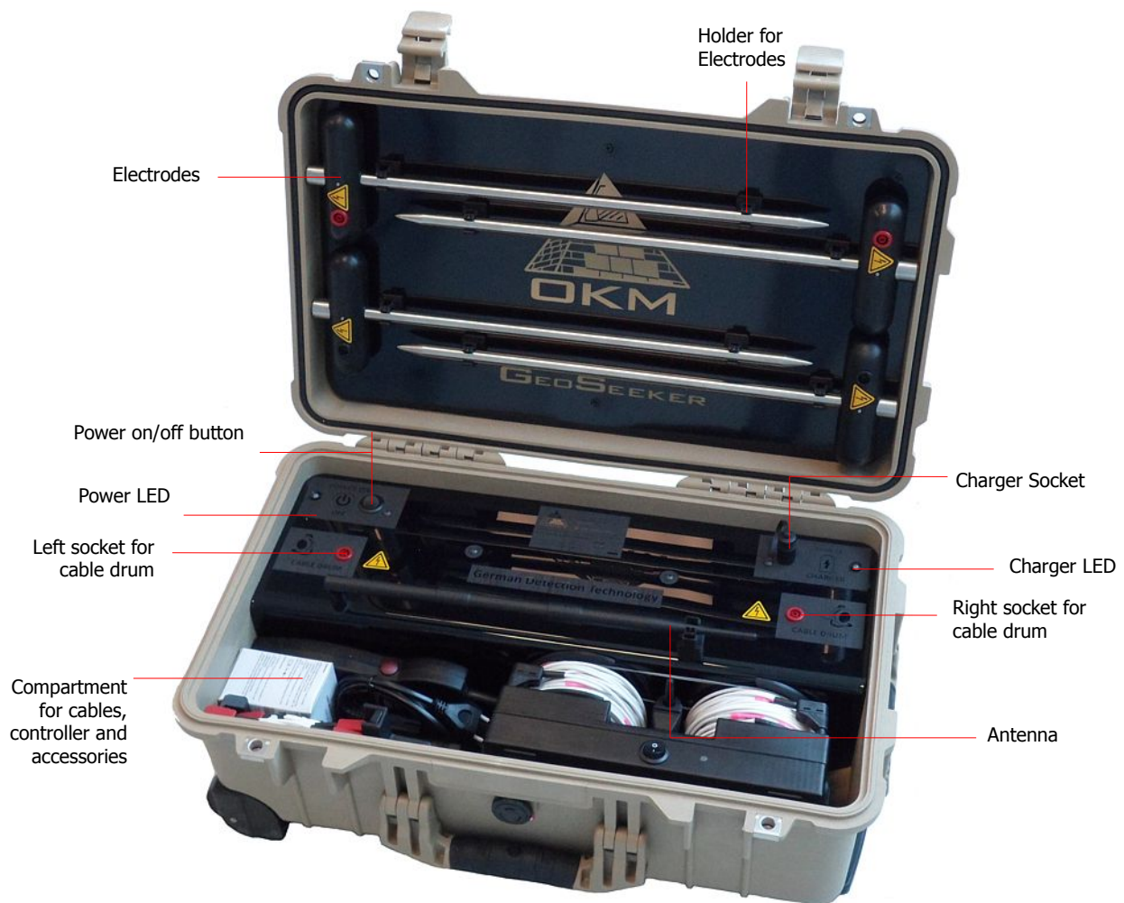
Figure 4.6: Control elements of the Power Box
