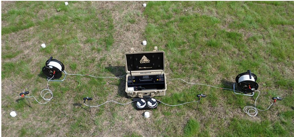
Figure 7.6: Arrangement of electrodes during Active Scan (Accurate)
