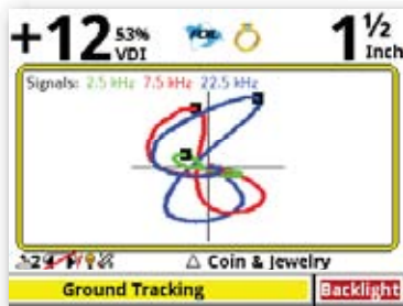
Typical Poor Quality Alloy
