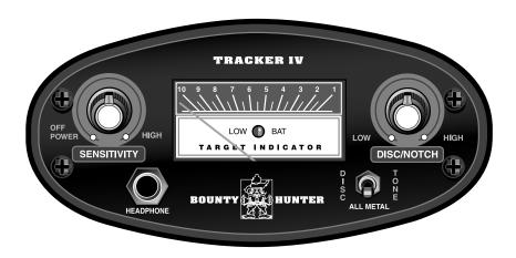
For maximum performance, operate with the sensitivity as high as possible. The sensitivity can generally be set higher when operating in Full Discriminate (DISC) or Tone Discriminate (TONE) modes.
