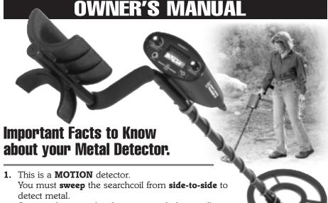
A motionless searchcoil over a metal object will not result in detection.
