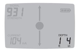
The weaker the signal strength, the less reliable the depth indicator. For this reason, depth readings for inductively located utilities will tend to be less accurate than conductively located ones.
