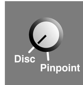
The Excalibur can operate in two different modes. This control selects either Disc (Discriminate) or Pinpoint mode.
